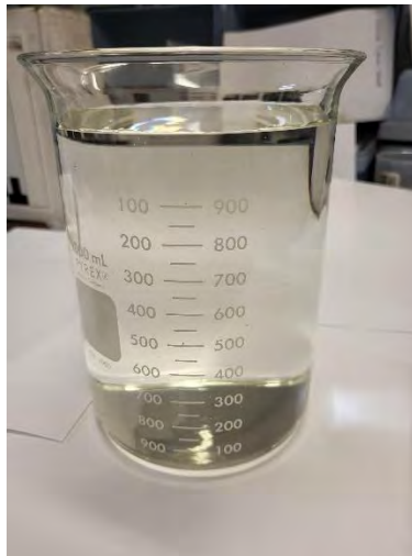
Figure 2. Composite Backwash Waste Sample (12/3/2021; 1.65 NTU)
