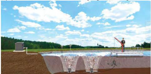
The aerators are placed into position from a floating vessel. Air is fed to manifolds on shore via a header from the blower. Each manifold port features a ball valve linking to the aerators by weighted air hose allowing for individual aerator control.
